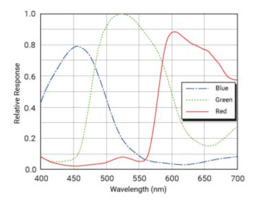
The spectral response curves exclude lens characteristics, light source characteristics, and IR cut filter characteristics.
