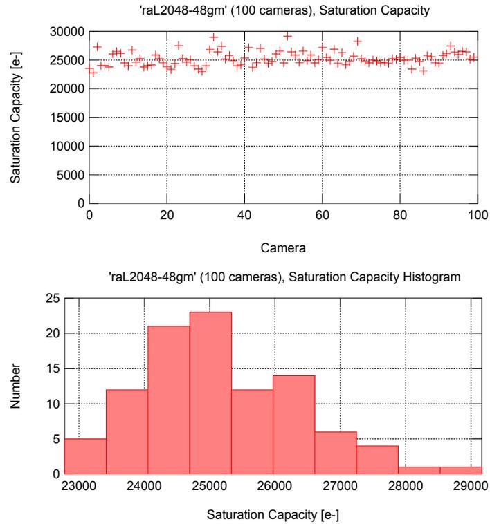
Figure 6: Saturation Capacity
